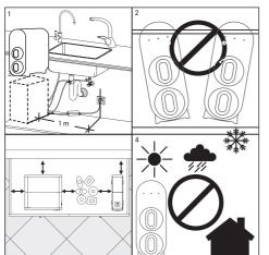
ATTENTION: The equipment must not be installed next to a heat source or directly receiving a flow
