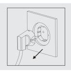
Read the sectionINTERFACE of the Technical Sheet. In case of anomaly, contact the SAT and proceed as indicated: Close the inlet valve. Open the tap to depressurize the system and unplug the plug.
