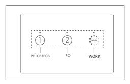
The equipment includes an intelligent faucet that will indicate by means of an LED the need to replace any of the cartridges or a malfunction of the system.
