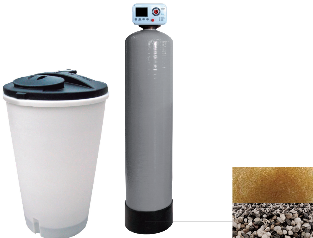
The silex base with different grain sizes optimises, the water flow, thus improving the regeneration process.
