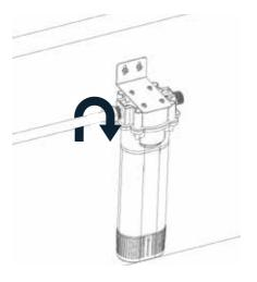
Install the water outlet tube in the direction shown in the diagram and ensure it is properly connected.
