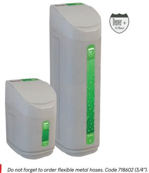
System is composed by a GRP bottle with top and bottom distributors and polyethylene cabinet. WS180-HE valve, electronic programmed, delayed regeneration with day override. Noryl male connection (size depending on model). Brine valve included in the cabinet. Isolation by-pass and hardness mixer included. **Specifications:** Min. pressure: 2.5 kg/cm<sup>2</sup>. Max. pressure: 8.5 kg/cm<sup>2</sup>.
