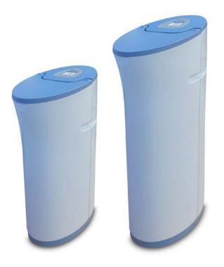
New generation high efficiency water softener with an innovative design and UpFlow regenerations. Cabinet composed by two independent bodies; resin vessel is completely isolated from brine tank. It's possible to install both parts as independent bodies. This system is composed of a GRP vessel with top and bottom distributors and polyethylene cabinet.
