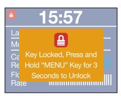
To unlock the programmer, press the 'MENU' button during 3 seconds.
