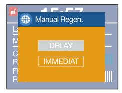
By pressing the 'SET/REGEN' button, the user can select the type of regeneration and with the 'MENU' button, the user can trigger the regeneration.
